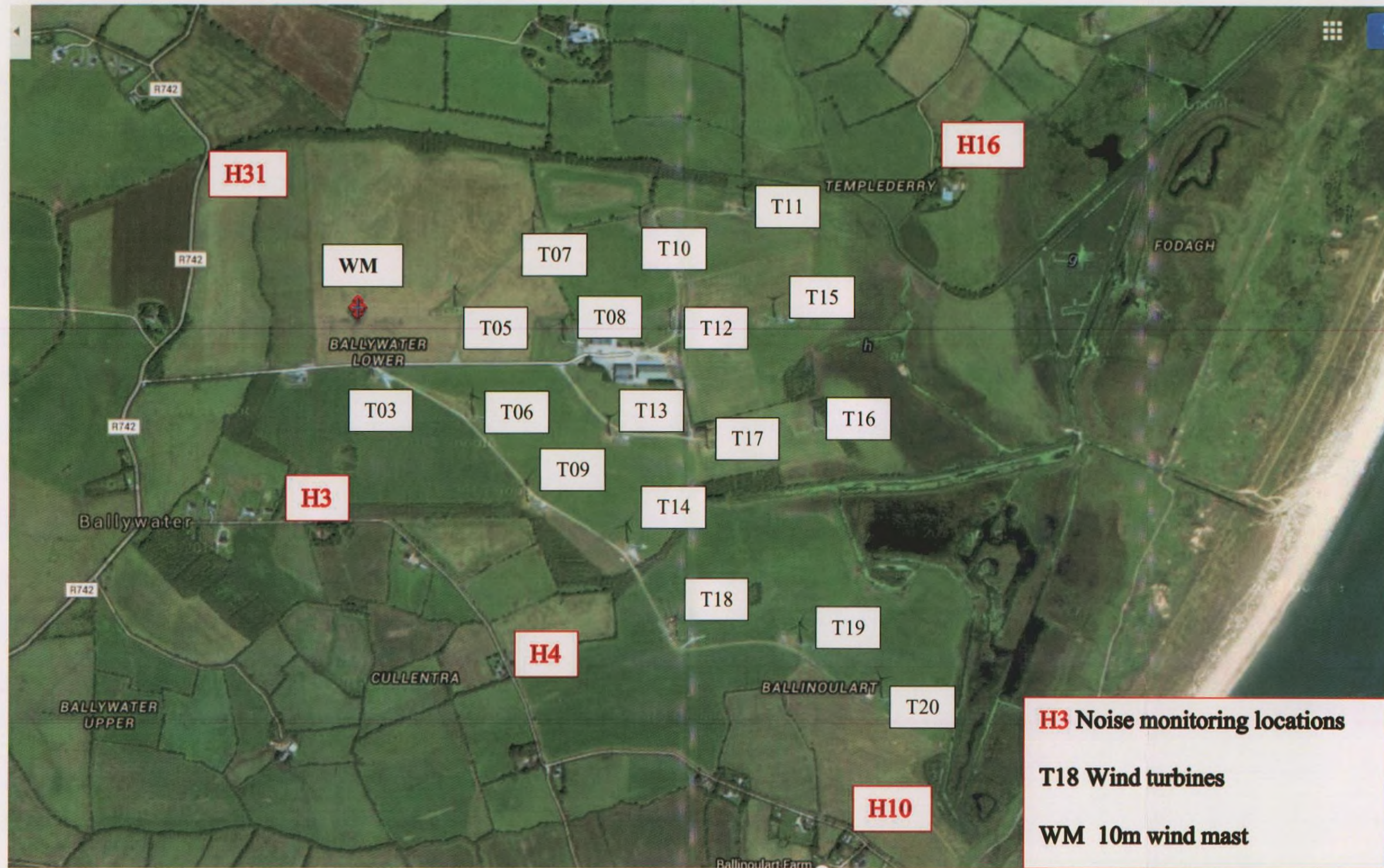
Figure 1 – As Constructed Turbine Locations and Noise Monitoring Locations
